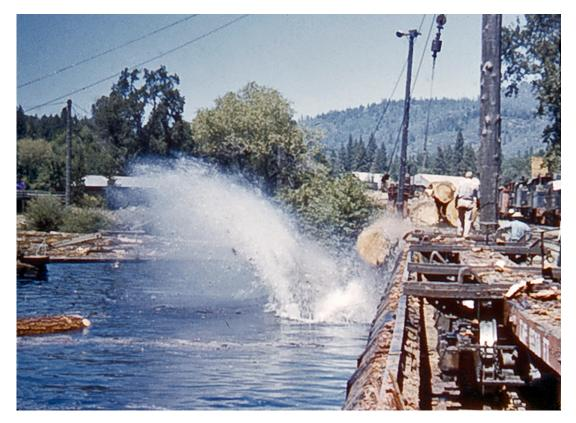
The second cable to the winch house could be seen in this photo. It was used to move a "traveler" along a fixed cable between the two spar poles so that the dumping setup was always over the car to be unloaded. It also was used in connection with the dumping cable to move the cars along the level track and even move them fast enough so they all would roll on to the tail track that curved
