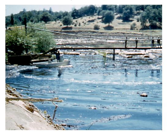
We also watched the pond boat in action, "herding" logs around the pond and away from the dumping area.
