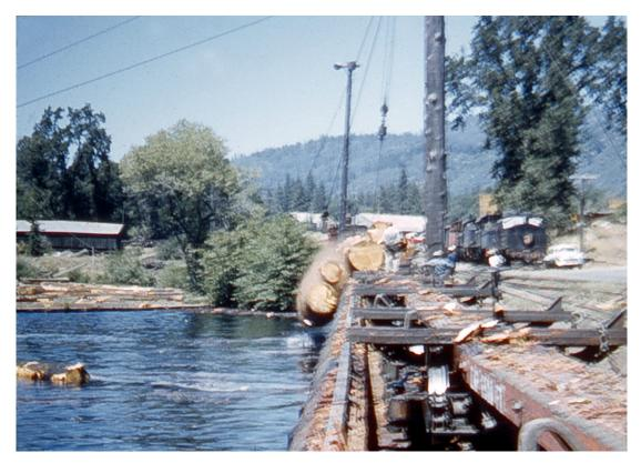
I went over to the end of the log pond brow nearest to the burner to watch the dumping. The concrete brow of the pond had a railroad rail mounted along its length. By design, the outer ends of the bunks of the log cars rested on this rail, thus keeping the cars from tipping as the logs were rolled off. The hook and block of the tripled dumping cable could
