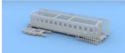
Coaches 19-22 built 1879 as first class cars. Duckbill roof.
